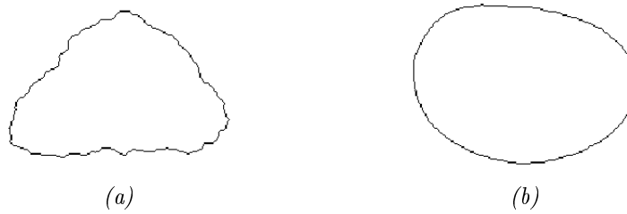
Fig. 2. Profile of rock fragments with roundness values of (A) 0.1 and (B) 0.9.
