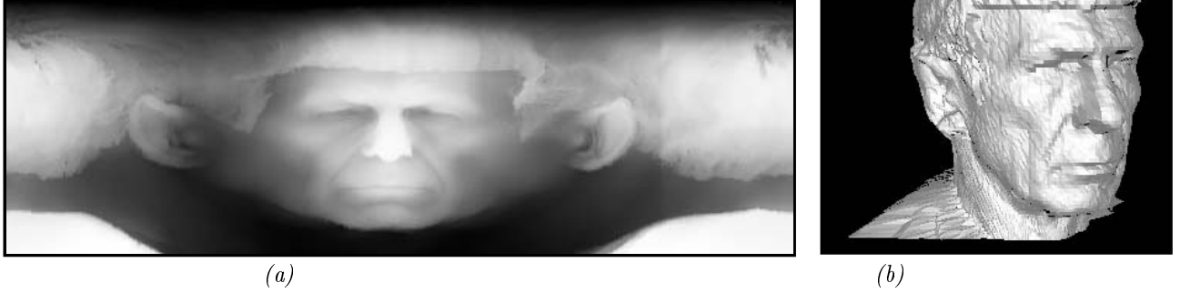
Figure 1 : (a) Depth of face parameterized as f(\theta, y) (Leonard Nimoy as Spock), (b) rendered polygonal model of face composed from coarse sampling of depth data.
